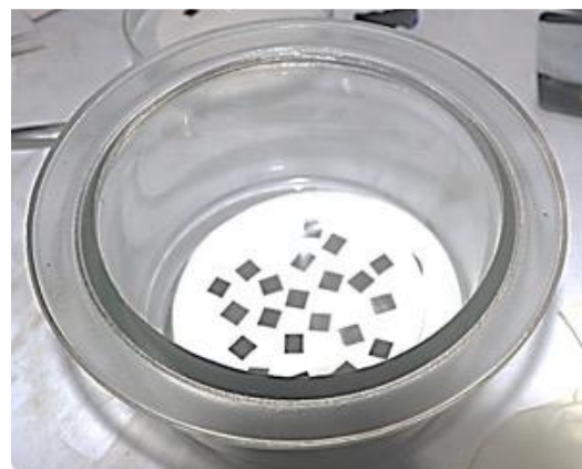
Figure 6 Mild steel specimen kept in a desiccator to avoid contamination.
