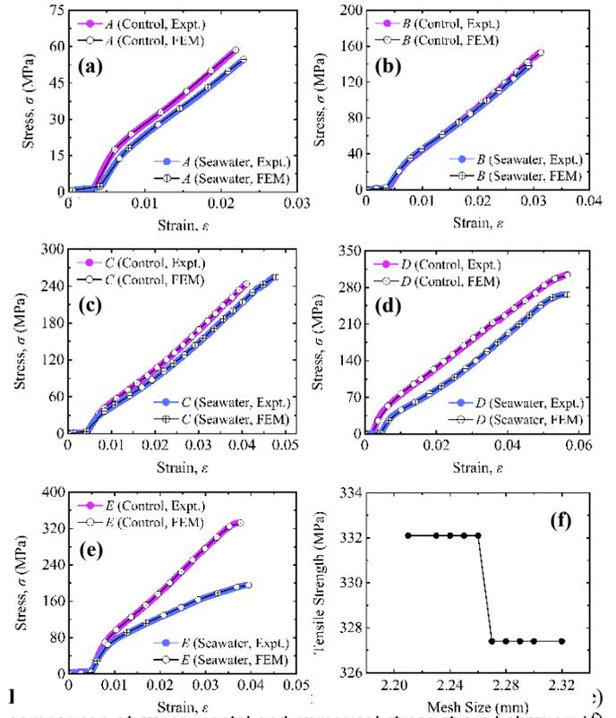
**Figure 3.** Comparison of experimental and numerical stress-strain behavior; (f) mesh convergence analysis for the numerical tensile test.
