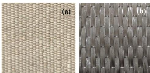
**Figure 1.** Reinforcements used: (a) JUCO fabric; (b) carbon fabric.
