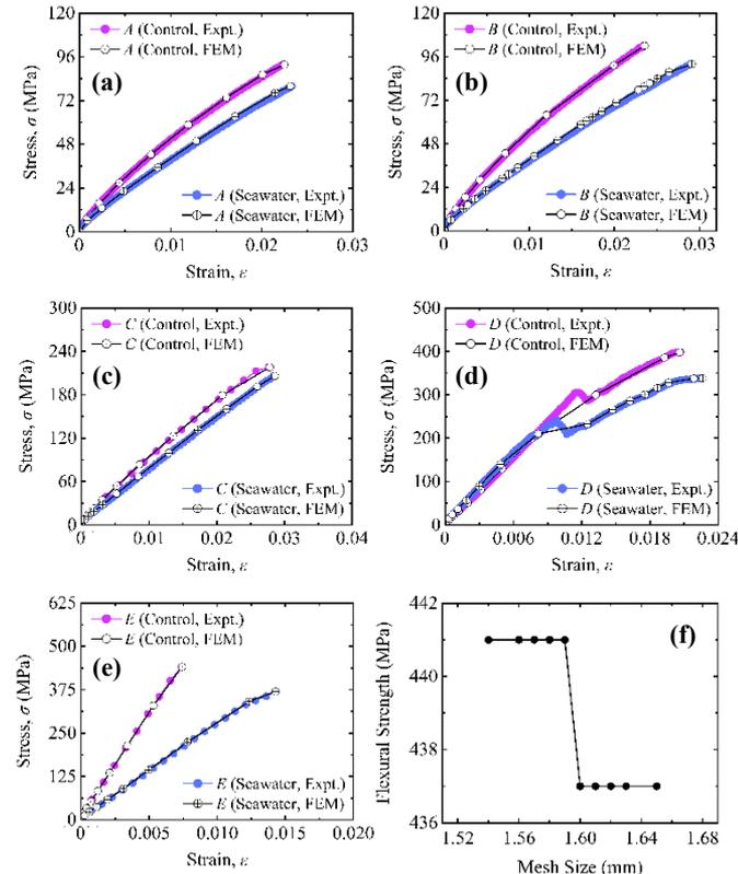
Figure 6. The validation of the flexural test results by FEM: (a)-(e) comparison of experimental and numerical stress-strain behavior; (f) mesh convergence analysis for the numerical flexural test.
