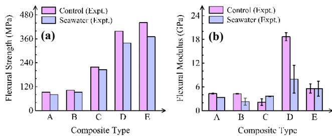
Figure 5. Effects of seawater aging on the flexural characteristics of the fabricated composites: (a) flexural strength; (b) flexural modulus.
