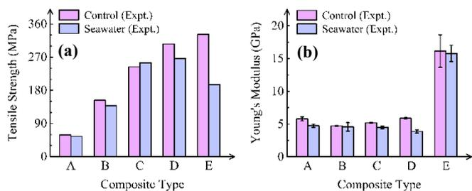
**Figure 2.** Effects of seawater aging on the tensile characteristics of the fabricated composites: (a) tensile strength; (b) Young’s modulus.
