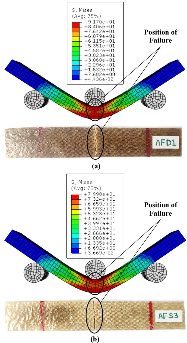
Figure 7. Von-Mises flexural stress distribution (FEM) and fractured specimen (expt.): (a) A-type (control); (b) A-type (seawater).
