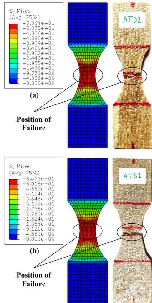
**Figure 4.** Von-Mises tensile stress distribution (*FEM*) and fractured specimen (expt.): (a) *A*-type (control); (b) *A*-type (seawater). the tensile strength of the JUCO composite as 49.66 MPa after aging in seawater. The tensile strength for the aged specimen
