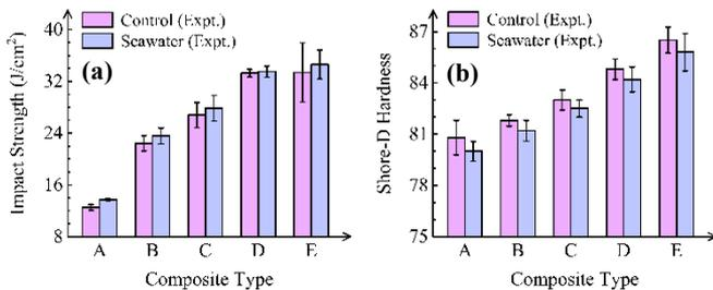
**Figure 8.** Effects of seawater on the impact and hardness properties of the fabricated composites: (a) impact strength; (b) hardness.
