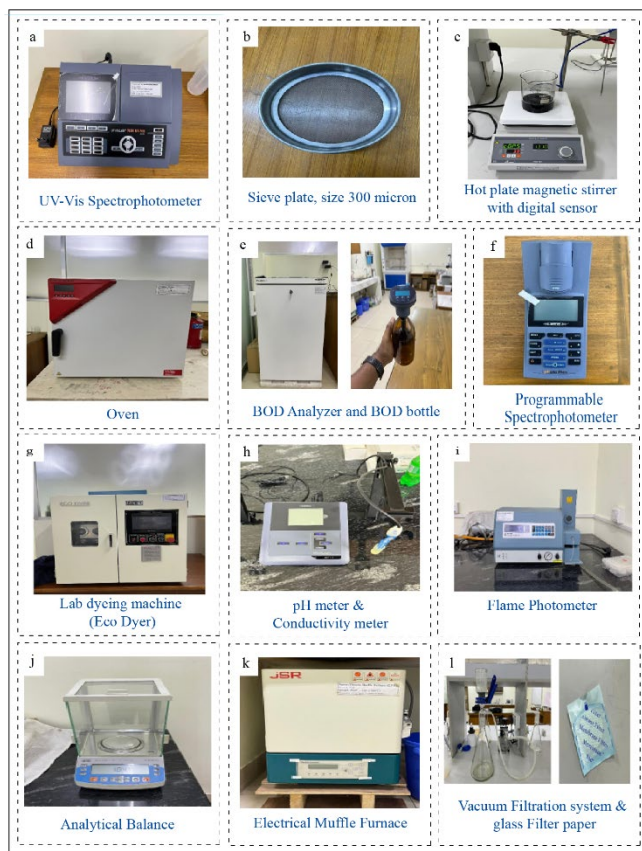
Figure 2. Instruments and equipment used: (a) UV–Vis spectrophotometer, (b) 300 \mu\text{m} sieve plate, (c) hot plate magnetic stirrer, (d) oven, (e) BOD analyzer and bottle, (f) programmable spectrophotometer, (g) lab dyeing machine, (h) pH and conductivity meter, (i) flame photometer, (j) analytical balance, (k) muffle furnace, and (l) vacuum filtration system with glass filter paper.
